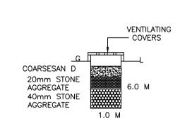
CROSS SECTION OF RAIN WATER HARVESTING WELL. ( DRAWING NOT TO SCALE. )
